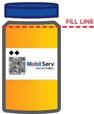
Secure the cap to the sample bottle. Visually inspect the sample for particulate, water or other contaminants.
